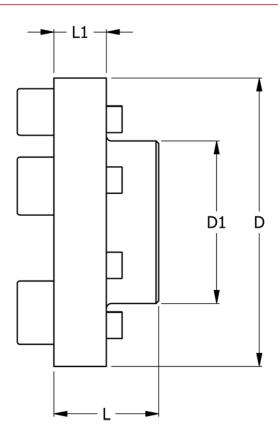
$\begin{array}{lll} D & = 350 \\ D1 & = 230 \\ L & = 140 \\ L1 & = 51 \\ Max bore & = 140 \\ Torque (N m) = 7700 \end{array}$
